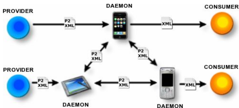
Fig. 1. Overview of the P2 system architecture with multiple provider and consumer nodes interconnected through the distributive P2 daemon network
